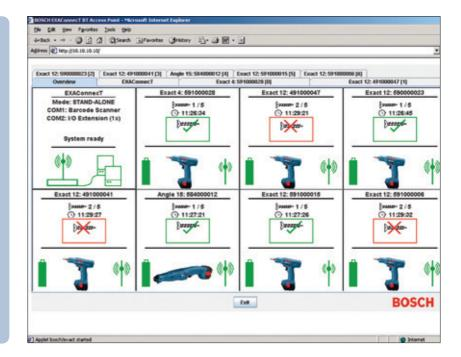
Clicking on the 'EXAConnecT' tab shows the detailed data for up to seven BT-EXACT screwdrivers in real time. The system can display extensive data such as BT-EXACT screwdriver name, date, time of event, screw runtime, direction of rotation, error messages, work progress and additional input data (such as barcode scans or sequence numbers).
