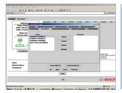
The system has separate configuration windows for the EXAConnecT controller and the BT-EXACT screwdrivers. The configuration screen shows part of the EXAConnecT configuration menu. The system can be password protected to prevent unauthorised use.
