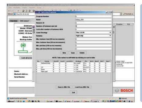
The screwdriver configuration menu on the left controls everything from screw count to rework strategy to data output choices. The BT-EXACT screwdriver and the EXAConnecT controller can be configured to send and receive data from a variety of systems, including a host ethernet system, PLC systems, barcode scanners or our digital I/O module.
