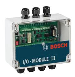
The digital I/O module takes its power from the EXAConnecT controller and receives its screwdriving data from the controller's RS 422 interface. The module has 16 inputs and outputs for exchanging data with a PLC. Configuration is done via the EXAConnecT software (in a web browser).
