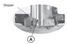
This portion of the stopper should be 0 mm to 0.5 mm ahead of the optical axis of the sensor when viewed from above. (The bit guide does not need to be removed.)
